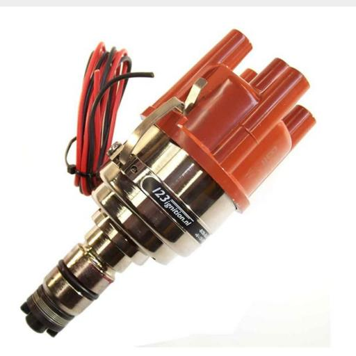
The Historic Production Based Eligibility Committee (HPBEC) has researched the "123 Distributor" and found that these are a full electronic ignition system completely housed within the distributor body. The electronic ignition system controls the ignition advance curve which is programmable.
