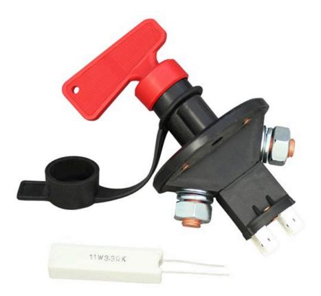
To properly isolate your battery from the ignition as well as the alternator, you need a switch with more than two posts. A lot of the popular car parts retailers sell the 2 post switches as battery isolation switches but they are not really doing that job.
